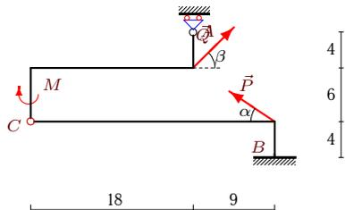
$$P = 30 \text{ кН}, Q = 40 \text{ кН}, \alpha = 30^\circ, \\ \beta = 45^\circ, \rho = 5 \text{ кН/м}, M = 110 \text{ кНм}.$$
