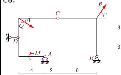
$$P = 20 \text{ кН}, Q = 30 \text{ кН}, \alpha = 60^\circ, \\ \beta = 30^\circ, \rho = 3 \text{ кН/м}, M = 70 \text{ кНм}.$$
