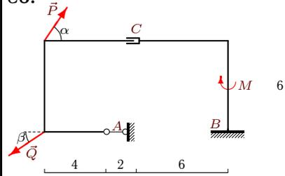
$$P = 20 \text{ кН}, Q = 30 \text{ кН}, \alpha = 60^\circ, \\ \beta = 30^\circ, \rho = 6 \text{ кН/м}, M = 60 \text{ кНм}.$$
