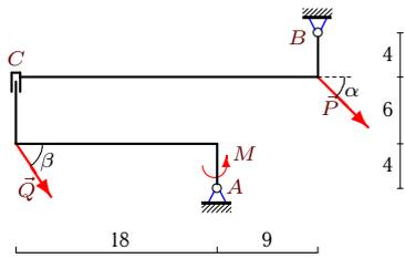
$$P = 60 \text{ кН}, Q = 70 \text{ кН}, \alpha = 45^\circ, \\ \beta = 60^\circ, \rho = 2 \text{ кН/м}, M = 30 \text{ кНм}.$$
