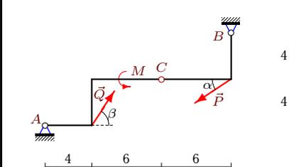
$$P = 10 \text{ кН}, Q = 20 \text{ кН}, \alpha = 30^\circ, \\ \beta = 60^\circ, \rho = 1 \text{ кН/м}, M = 70 \text{ кНм}.$$
