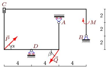
$$P = 60 \text{ кН}, Q = 70 \text{ кН}, \alpha = 45^\circ, \\ \beta = 60^\circ, \rho = 4 \text{ кН/м}, M = 10 \text{ кНм}.$$
