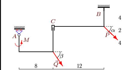
$$P = 60 \text{ кН}, Q = 70 \text{ кН}, \alpha = 45^\circ, \\ \beta = 60^\circ, \rho = 6 \text{ кН/м}, M = 40 \text{ кНм}.$$
