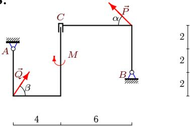
$$P = 60 \text{ кН}, Q = 70 \text{ кН}, \alpha = 45^\circ, \\ \beta = 60^\circ, \rho = 2 \text{ кН/м}, M = 50 \text{ кНм}.$$
