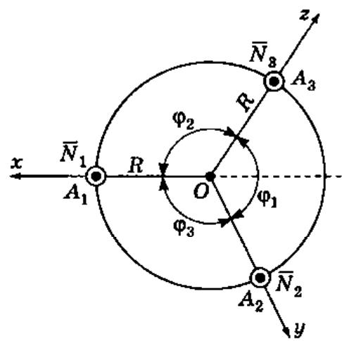
$$\begin{cases} N_2 R \sin(180^\circ - \varphi_3) - N_3 R \sin(180^\circ - \varphi_2) = 0, \\ -N_1 \cdot R \sin(180^\circ - \varphi_3) + N_3 \cdot R \sin(180^\circ - \varphi_1) = 0, \\ -N_2 \cdot R \sin(180^\circ - \varphi_1) + N_1 \cdot R \sin(180^\circ - \varphi_2) = 0. \end{cases}$$
