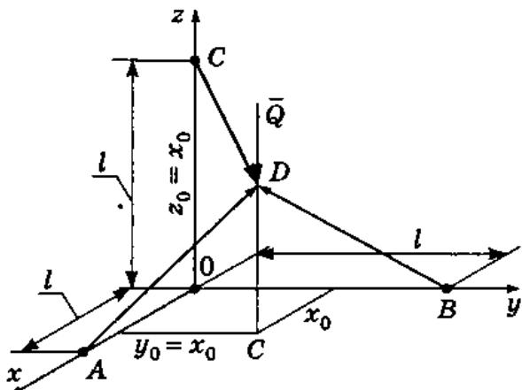
$$\Delta = \begin{vmatrix} x_0 - l & x_0 & x_0 \\ x_0 & x_0 - l & x_0 \\ x_0 & x_0 & x_0 - l \end{vmatrix} = l^2(3x_0 - l).$$
