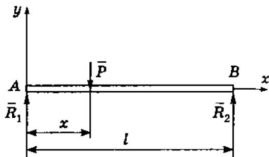
$$\begin{cases} R_2 l - Px = 0, \\ R_1 - P + R_2 = 0 \end{cases} \Leftrightarrow \begin{cases} R_2 = P \frac{x}{l}, \\ R_1 = P - R_2 \end{cases} \Leftrightarrow \begin{cases} R_2 = P \frac{x}{l}, \\ R_1 = P \frac{l-x}{l}. \end{cases}$$
