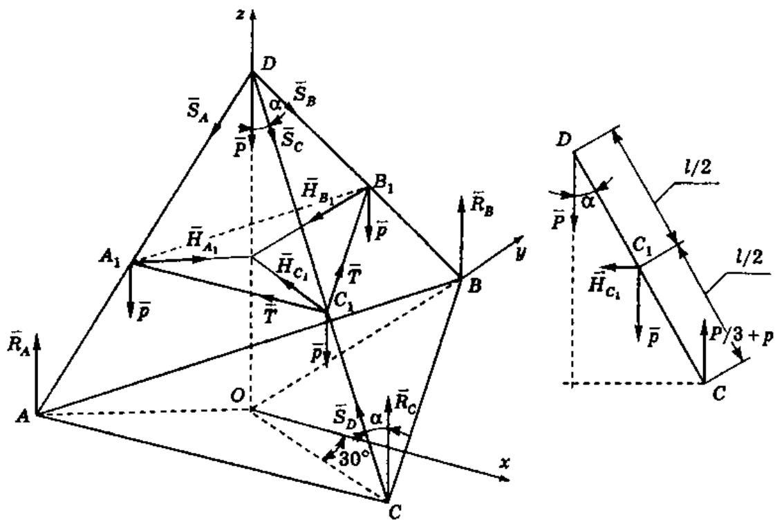
$$2T \cos 30^\circ = H_{C_1} \Rightarrow T = \frac{H_{C_1}}{2 \cos 30^\circ} = \frac{\frac{P\sqrt{2}}{3} + \frac{p}{2}\sqrt{2}}{2 \frac{\sqrt{3}}{2}} = \frac{(2P+3p)\sqrt{2}}{6\sqrt{3}} = \frac{2P+3p}{18}\sqrt{6}.$$
