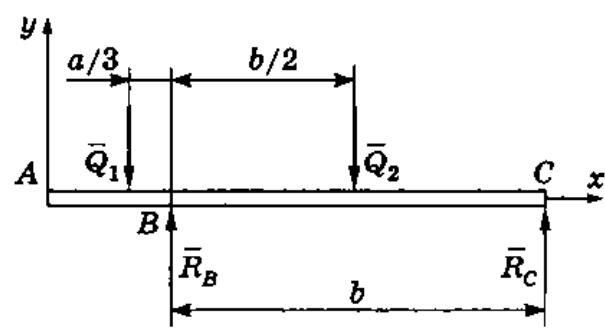
$$\begin{cases} \bar{Q}_1 \cdot \frac{a}{3} - \bar{Q}_2 \cdot \frac{b}{2} + R_C \cdot b = 0, \\ -\bar{Q}_1 + R_B - \bar{Q}_2 + R_C = 0. \end{cases}$$
