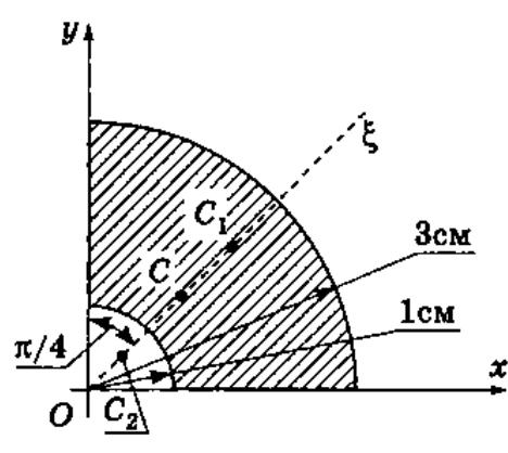
$$S_2 = \frac{1}{4} \pi R_2^2, OC_2 = \frac{2}{3} R_2 \frac{\sin \frac{\pi}{4}}{\frac{\pi}{4}} = \frac{4\sqrt{2}}{3\pi} R_2.$$
