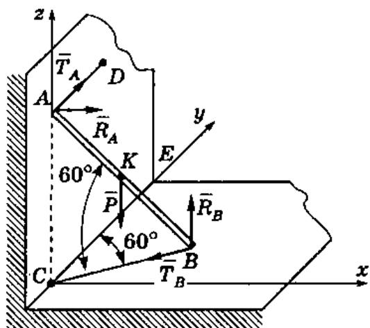
$$\begin{cases} R_A - T_B \cos 30^\circ = 0, \\ T_A - T_B \cos 60^\circ = 0, \\ R_B - P = 0, \\ P \cdot \frac{AB}{2} \cos^2 60^\circ - R_B AB \cos^2 60^\circ + R_A \cdot AB \cos 60^\circ = 0. \end{cases}$$
