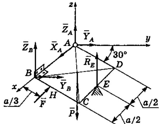
$$\begin{cases} X_A - F = 0, \\ Y_A + Y_B + R_E \sin 30^\circ = 0, \\ Z_A + Z_B - P + R_E \cos 30^\circ = 0, \\ R_E \cdot a - P \cdot 0,5 \cdot a \cos 30^\circ = 0, \\ -Z_B \cdot a + F \cdot \frac{a}{3} \sin 30^\circ + P \cdot \frac{a}{2} \cos 30^\circ - R_E \cdot \frac{a}{2} \cos 30^\circ = 0, \\ Y_B \cdot a + F \cdot \frac{a}{3} \cos 30^\circ + R_E \sin 30^\circ \cdot \frac{a}{2} = 0. \end{cases}$$
