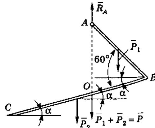
$$-\bar{P}_1 \frac{1}{2} AB \cos(60^\circ - \alpha) + \bar{P}_2 \left[ \frac{1}{2} BC \cos \alpha - AB \cos(60^\circ - \alpha) \right] = 0.$$
