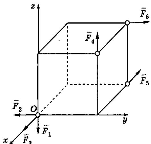
$$\left\{ \begin{array}{l} V_x = \sum_{k=1}^6 F_{kx} = F_3 - F_5 = 0, \\ V_y = \sum_{k=1}^6 F_{ky} = F_6 - F_2 = 0, \\ V_z = \sum_{k=1}^6 F_{kz} = F_4 - F_1 = 0, \\ M_x = \sum_{k=1}^6 M_x(\bar{F}_k) = F_4 \cdot a - F_6 \cdot a = 0, \\ M_y = \sum_{k=1}^6 M_y(\bar{F}_k) = 0 = 0 \text{ (выполняется тождественно)}, \\ M_z = \sum_{k=1}^6 M_z(\bar{F}_k) = F_5 \cdot a - F_6 \cdot a. \end{array} \right.$$
